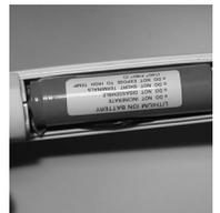
Fig 8: Seat the battery in the compartment, slide the cover in place and replace the screw.
