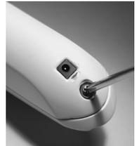
Fig 5: Remove screw.
