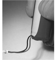
Fig 6: Bend replacement battery wire to facilitate positioning of the connector.
