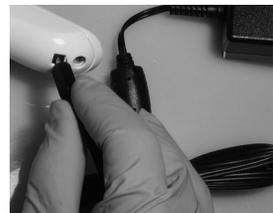
Fig. 2: Plug charger into square socket on the bottom of the handle.
